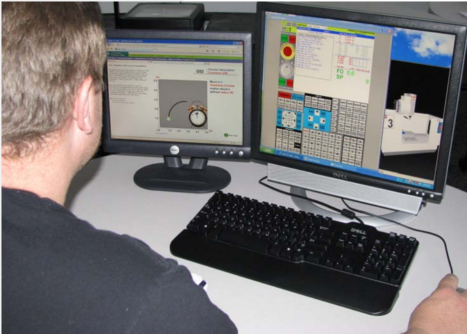
Instructors and students benefit from online interactive learning content, exercises, assessments and virtual CNC panels and 3D machines that run actual M&G code programs.
